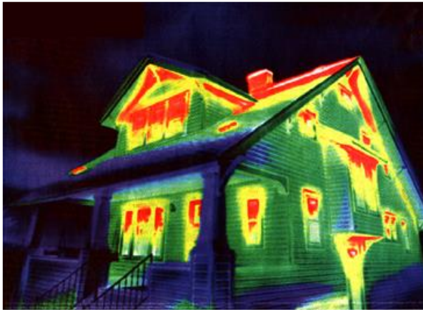
IR image of conductive losses in home
